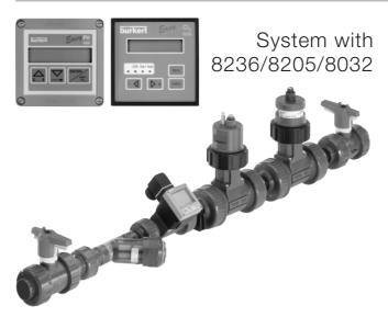
This chlorine control system for disinfectant measuring and dosage is designed for swimming pool applications, drinking, process and waste water treatment. Thanks to the Easy LINK with Burkert valves, the system provides an excellent low Total Cost of Ownership. The system consists of a chlorine controller (type 8236), a flow sensor/switch (type 8032), a pH-transmitter (type 8205), a filter and two ball valves (type 2657).
